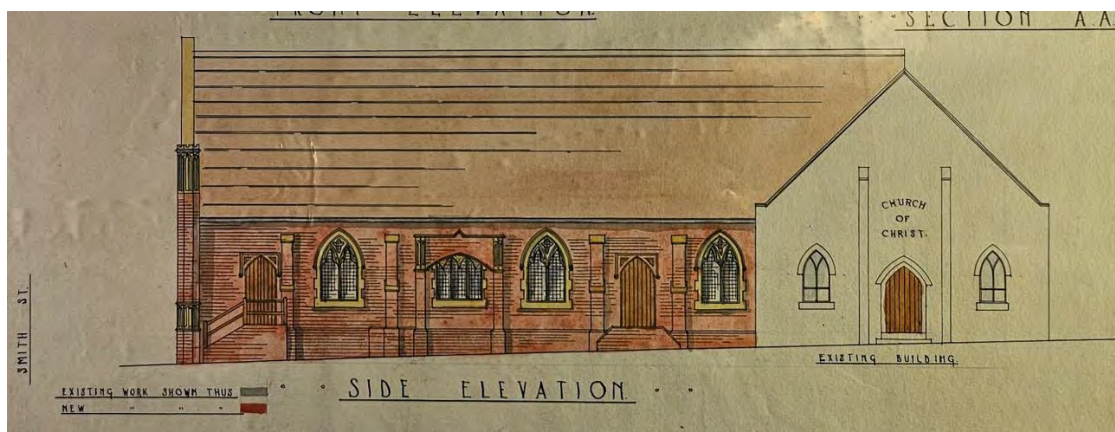
Figure 4 Side (south) Elevation of the Church of Christ, Thornbury, 1926, by Victor G Cook showing the Church of Christ constructed in c 1922 without colour and the 1927 extension designed by Victor G Cook in colour. Source: State Library of Victoria.
