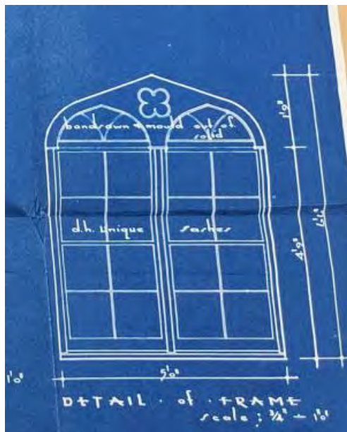
Figure 10 c 1953 detail of window frames on west elevation of the Church of Christ, Preston. Source: PROV VPRS 7882/P0001
