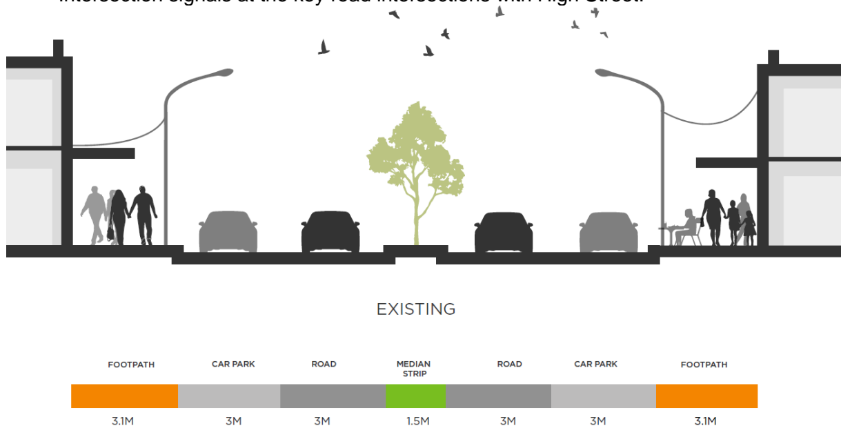
Figure 1 - Existing cross section of High Street
