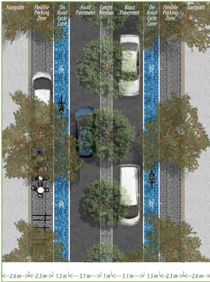
High Street - Concept Enlargement Plan Note: Bicycle lanes shown blue for illustration purposes only. They would be installed to relevant standards and not coloured as indicated.
