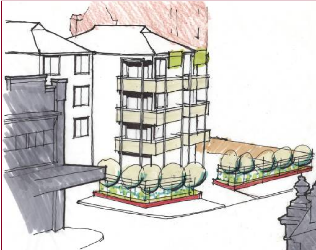
Indicative sketch of new façade to units at south east corner of James and High Street, illustrating how a new façade could be vertically incorporated into the existing units so as to improve amenity of site and surrounds.
